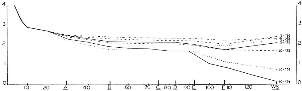
FIG. 2. Bog surface profiles, showing levels at the various dates surveyed. Permanent stations indicated by letters along the baseline. Vertical scale in feet, horizontal scale in meters.
